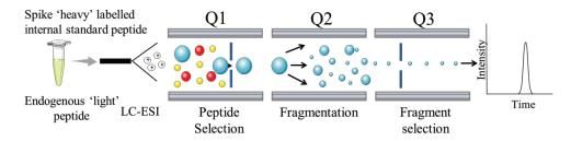
**Figure 3.2 Schematic workflow of SRM-based proteomic experiment.** A triple quadrupole (QQQ) mass spectrometer (Q-Trap). Figure modified from (186).
