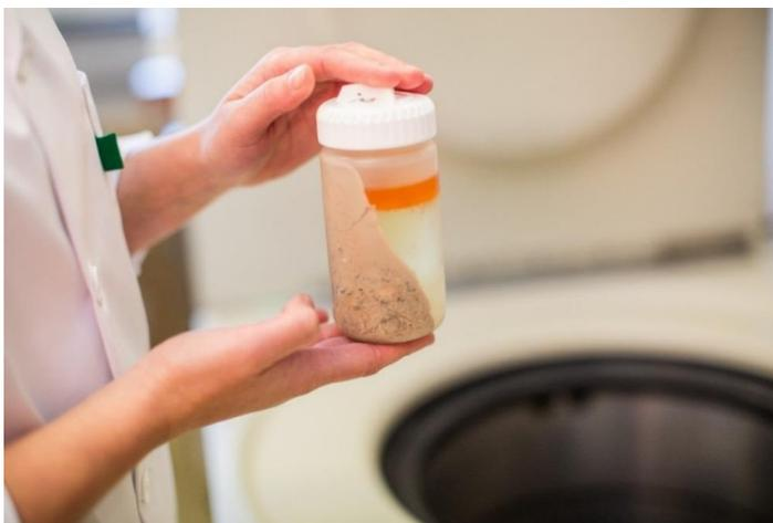
**Figure 6.** After centrifugal separation the hydrolyzed fish slurry were divided into a semi-solid layer at the bottom, water-soluble protein hydrolysates in the middle and an oil-layer on top. Photo by Øyvind Ganesh Eknes.
