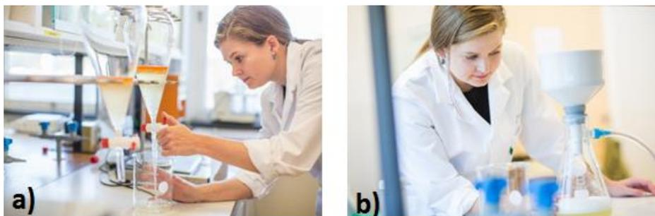
**Figure 7.** a) Separation of the lipid phase and water-soluble hydrolysate through a separation funnel, b) Filtering of the water-soluble protein hydrolysate over a Büchner filter. Photo by Øyvind Ganesh Eknes.
