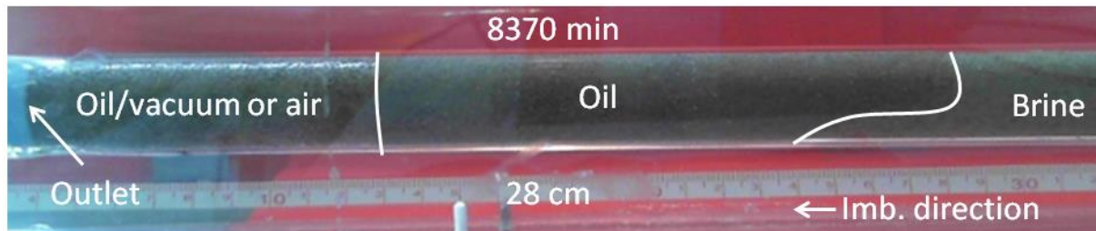
Figure 54: Front behaviour during spontaneous co-current imbibition where polymer was used as the wetting phase, whereas decane was used as the non-wetting phase. This picture shows the front behaviour after the filter was removed, during the later stages of the experiment.
