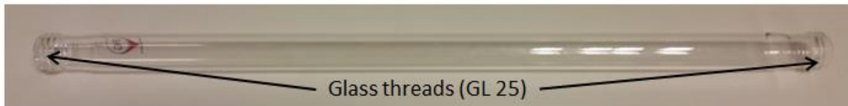
Figure 19: Imbibition tube made of glass used in experiments. 50 cm long with an internal diameter of 20.4 mm, and with glass threads (GL 25) at each end.
