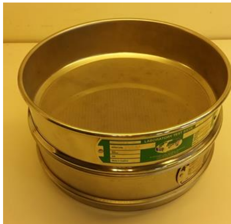
Figure 18: Geological sieves used during sieving of sand. One sieve had a mesh size of 250\text{ }\mu\text{m} , whereas the other had a mesh size of 212\text{ }\mu\text{m} .
