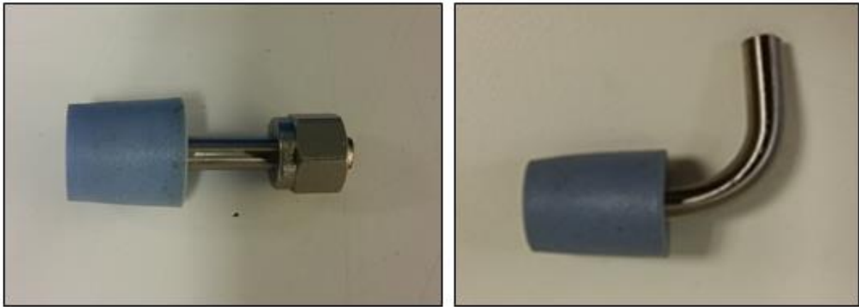
Figure 21: Conical rubber end pieces pierced with 1/4 inch stainless steel tubing. Left: straight end piece with Swagelok fitting. Right: 90° end piece.
