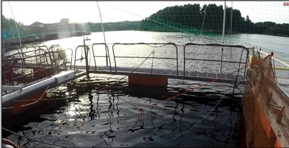
Figure 6. An experimental net-pen at the Austevoll Research Station. The dimensions are approximately 5x5x6.5 metres, with a pyramid-shaped base and a collection bag at the bottom for any dead fish.
