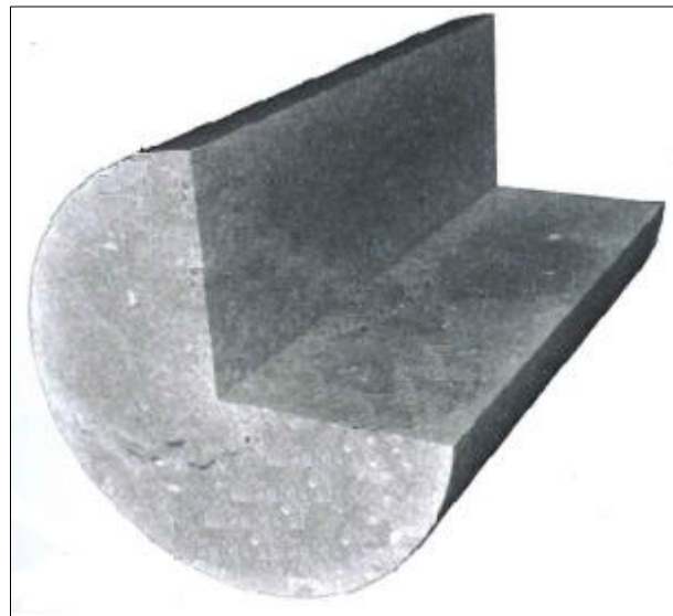
Figure 11: Three dimensional CT image of a water saturated Portland chalk core (Eide, 2011). Dark shade represents high-density areas where x-rays experienced significant attenuation whereas a lighter color indicates less dense material.
