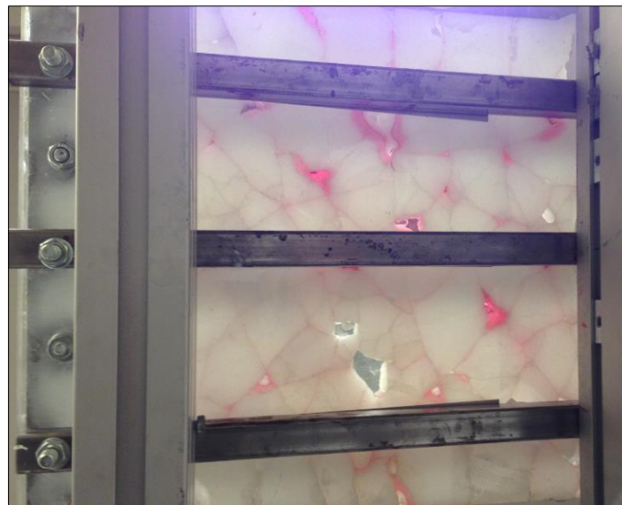
Figure 17: Photo of the fractured marble network after injection of a red contrast fluid. Although the majority of the fractures were narrow, some wide ones (seen with red contrast fluid) were included to make it possible to observe foam propagation and variation in foam quality during the experiments (Fernø et al., 2016).
