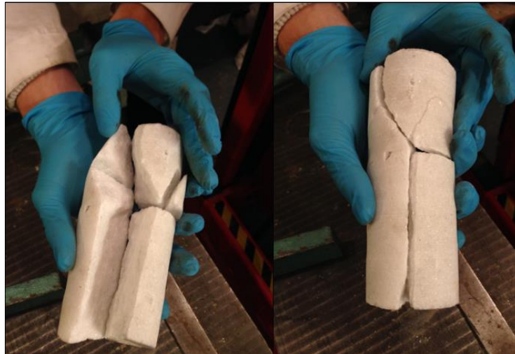
Figure 15: Fractured core sample. Remaining dust and debris were carefully brushed away before the pieces were puzzled together.
