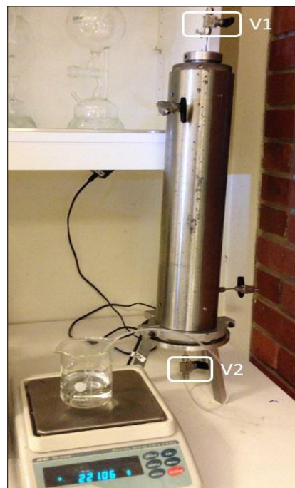
Figure 18: Photo of a vertically placed two-inch core holder during pore volume estimation using the saturation method. An upright position was used to fill the core with brine from the bottom and displace pockets of air.
