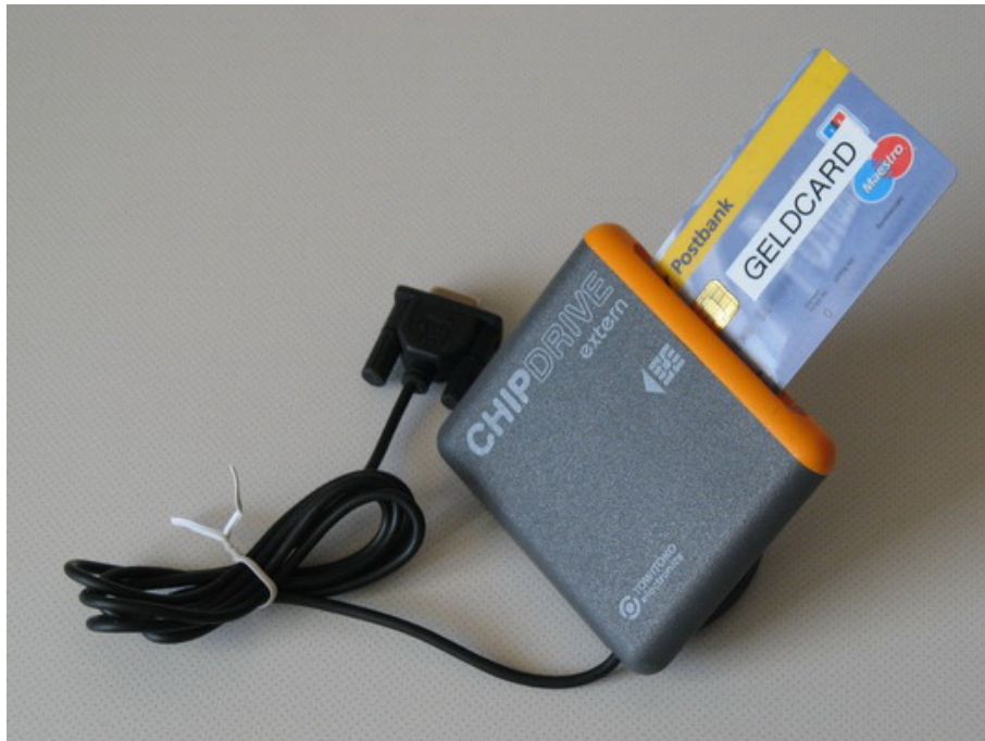
Figure 2.1: Contact smart card and reader.
