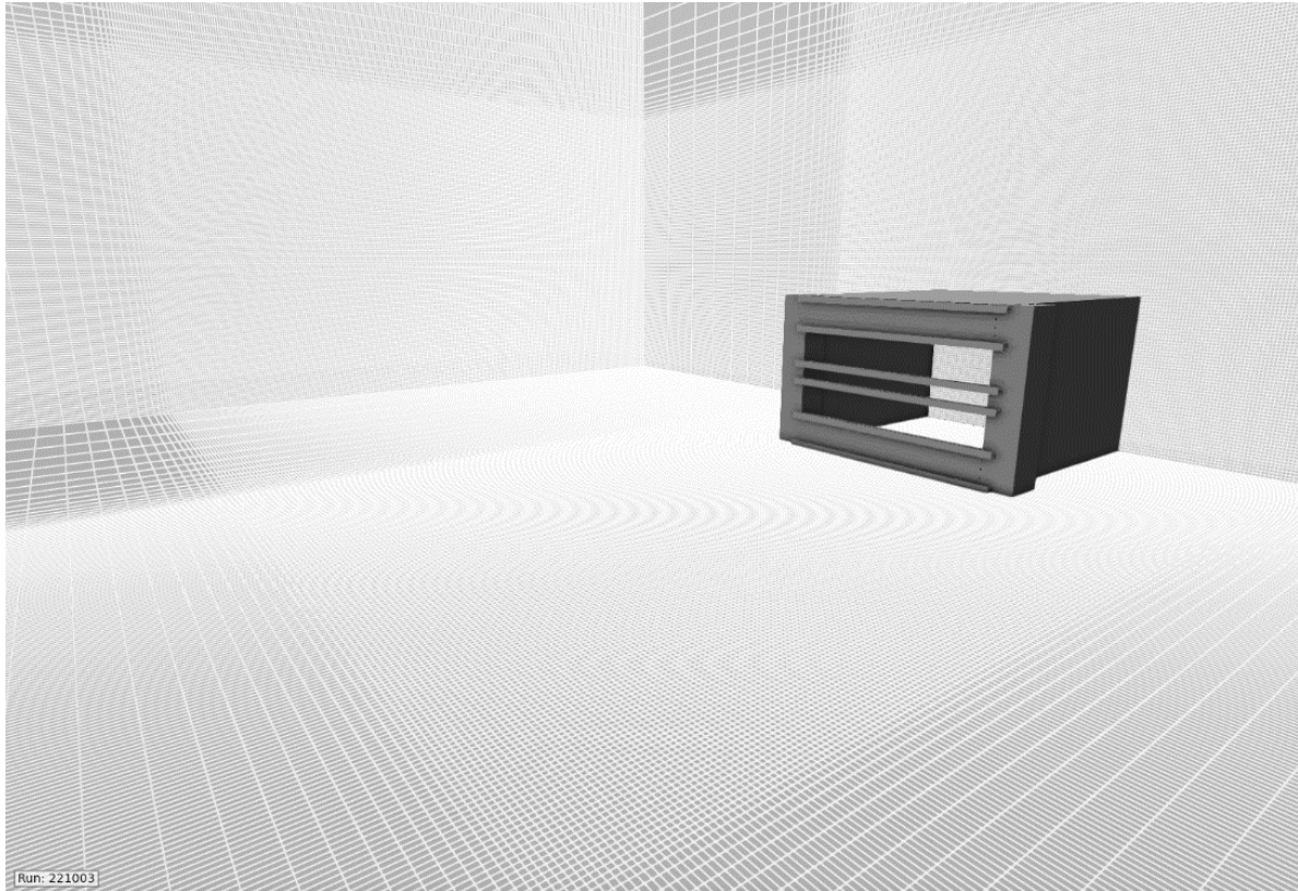
Figure 13: Graphical image of enclosure of 38,5 m 3 used in FLACS for simulations of experiments van Wingerden [12].
