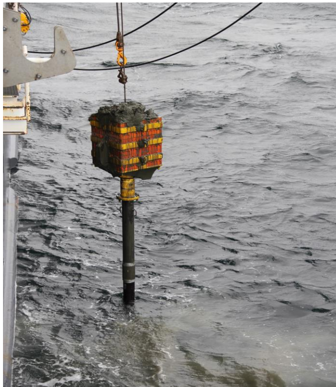
Figure 4.1.1. Picture of the calypso corer used on board F/F G. O Sars, taken during the Ice2ice cruise (Photo: Ida Synnøve Folkestad Olsen).
