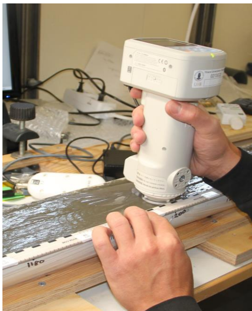
Figure 4-1-3. Picture taken during the ice2ice cruise showing color scanning of sediment with the use of a spectrophotometer (Photo: Ida Synnøve Folkestad Olsen)
