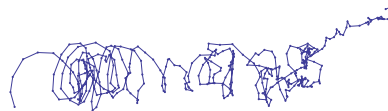
Figure 4.13: The particle in Figure 4.12 (b) has passed the turbulent region and continues spiraling in a slower and staggering manner.
