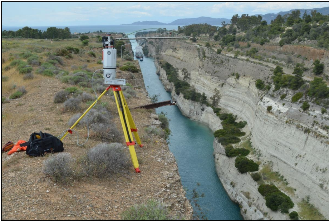
Fig. 3.1: Terrestrial LiDAR scanner (Riegl VZ-1000) used in the Corinth Canal. Photo taken by Martin Muravchik.
