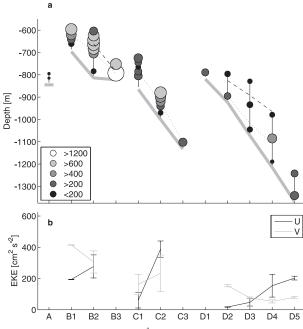
FIG. 6. (a) Mean EKE (cm s<sup>-1</sup>) obtained from Fourier analysis in the band of 2.5–5 days at mooring arrays A–D. The energy at a certain depth is proportional to the area of the circle centered at that depth. The mean position of the 3° (dotted) and 6.5°C (dashed) isotherms is indicated. Lack of an isotherm means that it is located above the uppermost recorder for more than 25% of the time. (b) Mean EKE above the bottom boundary layer (80 m) for the *u* and *v* components.
