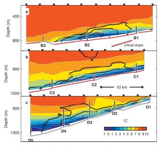
FIG. 2. Position and vertical extent of moorings superimposed on temperature (in color) and along-slope currents (black contours;  $m s^{-1}$ ) at time of deployment for (a) array B, (b) array C, and (c) array D. Black triangles mark the position of CTD/LADCP profiles. Vertical and horizontal scales in (b) are identical for all panels. The critical slope defined by Nof et al. (2002) is shown in (a). Eddies are expected to occur where the slope is subcritical (marked with red).
