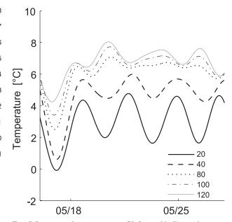
FIG. 5. Low-passed temperature at C3. Legend indicates the mean instrument level as height above bottom (m).
