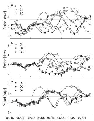
FIG. 14. Oscillation periods obtained from the located peaks in (a) u, (b) v, and (c) T. The gray line marks the 88-h period found by Geyer et al. (2006).
