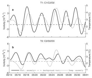
FIG. 10. Relative vorticity  $\xi$  anomaly from 100 mab (black line) and background vorticity (dashed line) and mean temperature anomaly from 30 mab (gray line) for mooring triangle (a) T1 (C1/C2/D2) and (b) T2 (C2/D2/D3).
