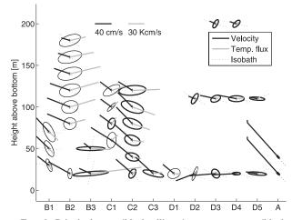
FIG. 8. Principal axes (black ellipses), mean currents (black lines), and temperature fluxes (gray lines) observed at the moorings. CW and CCW rotation of the velocity vector is indicated by thin and thick lines in the ellipse, respectively.
