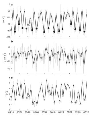
FIG. 3. Time series of (a) along-slope u and (b) across-slope v velocity and (c) temperature acquired by instruments 100 mab at D4 (bottom depth 1205 m). Hourly time series (gray) are low passed with a cutoff period of 48 h (black). Dominant subinertial oscillations (located by negative maxima in u, v, and T) are indicated by circles. The events marked by filled circles in (a) are included in the ensemble average (see section 3b).
