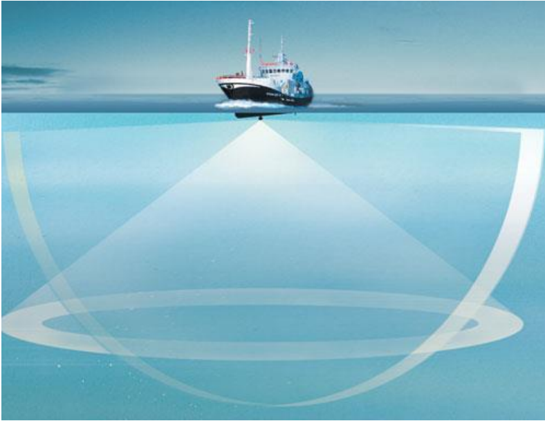
Figure 5, Picture of the two sonar fans from the SX90 sonar. The conical fan is an illustration of the beams' orientation in the horizontal mode, while the vertical aligned semicircle illustrates the orientation of the beams in the vertical mode. (SIMRAD. 322074/A 12.2011)
