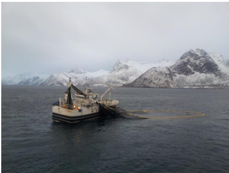
Figure 2. Photographic image showing the purse seiner F/V "Sjarmør" during the last stages of hauling a school of herring. Photo: Sindre Vatnehol.
