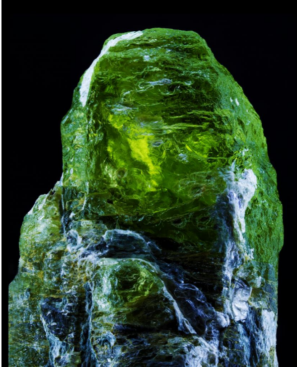
Figure 6.3.26: Transparent subhedral forsterite crystal approximately 4.5 cm high and 1.5 cm wide illustrating alteration from forsterite to talc.
