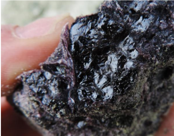
Figure 6.4.21: Subhedral magnesiochromite crystal in clinochlore matrix representing sample JVS 218A and JVS 218B.
