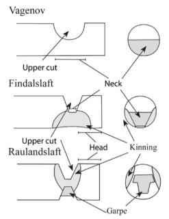
**Figure 7.** 'Vagenov', 'findalslaft' and 'raulandslaft' and the different parts of the notched joints.
