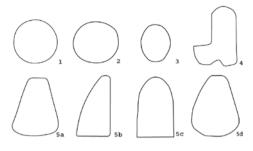
**Figure 4.** Sill beams with examples of different crosssections: 1. round, 2. flat-oval, 3. oval, 4. rectangular, 5a.-d. trapezoidal.
