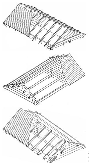
**Figure 12.** Different construction types of roofs. From the top: Collar rafter roof ('sperretak'), side purlin roof ('åstak'), and a combination of the two (After Godal 1994).
