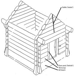
Figure 3. A log built building with the denomination of possible to determine the cross-section of some of the construction elements discussed in the article
