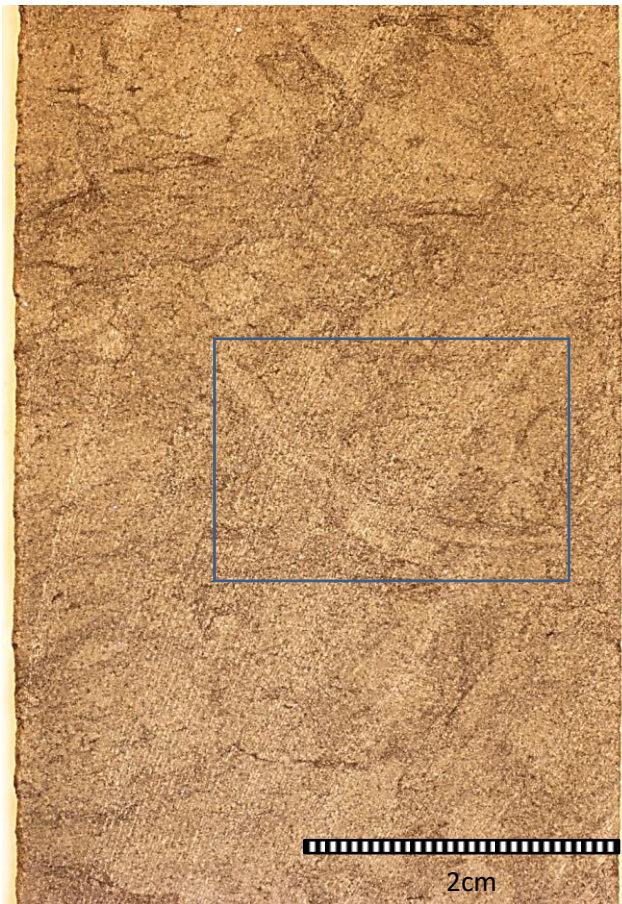
Figure 3.2: Vertical-section with Cylindrichnus concentricus , in well BH-10-2008, depth 873.75 m.
