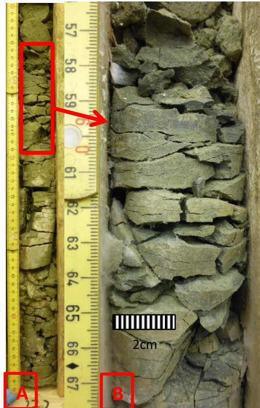
Figure 4.5: (A) a 50 cm bentonite layer occurs in Lithofacies F.4 in well BH-9-2006, depth: 272.50-273.00. (B) A close-up of the bentonite layer, depth: 272.56-272.68.
