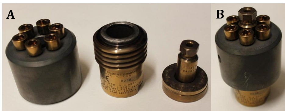
Figure 3.3 – A: Disassembled 25 mL Parr reactor. B: Assembled 25 mL Parr reactor.
