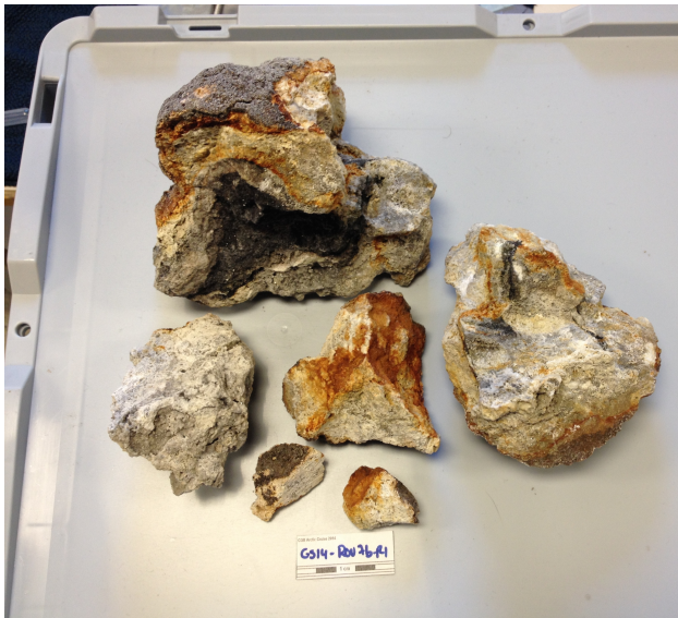
Figure 26: Picture of the sampled feeder system. In the big piece in the upper left of the frame it is clearly seen that there is a sharp contrast in colour between the outer parts that is light in colour, and the darker interior.
