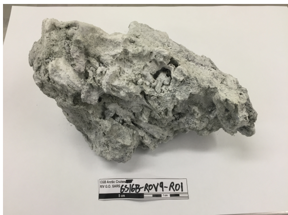
Figure 55: Picture of a fragment taken from the sampled active chimney. The sample has a light colour and is mainly composed of anhydrite.
