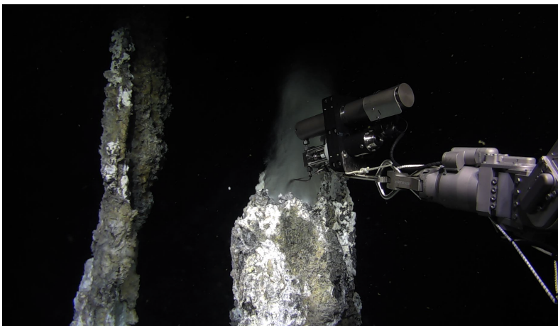
Figure 13: Picture of temperature probing and fluid collection from the active vent (GS16B-ROV9-R01). The vent was sampled with the use of the ROV grabbers.
