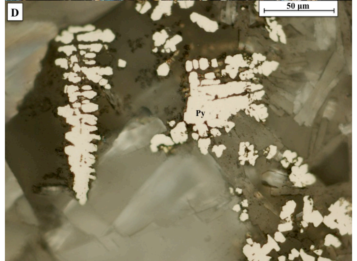
Figure 59: Picture A and B shows anhedral to subhedral tabular or acicular anhydrite crystals and patches of colloform silica. C and D show the sulphide assemblages found in the thin section, which is identical to that found in figure 57.
