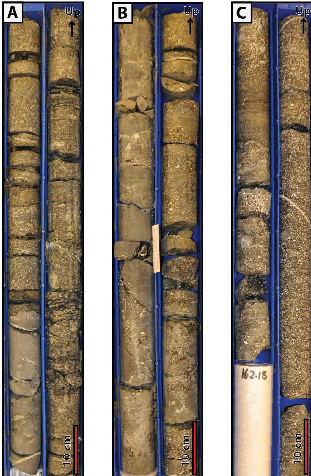
Figure 4.2: Figure displaying the different lithofacies observed in the core. (A) Matrix-supported hyaloclastite breccia (Group 1) and coherent lava flow facies. Note the irregular upper contact between the units in the lower left part of the figure. (B) Matrix-supported hyaloclastite breccia grading into clast-supported hyaloclastite breccia (from right to left in the picture). (C) Fine-grained hyaloclastite ash (dark area to the upper left) grading into more coarse-grained, matrix-supported hyaloclastite breccia (Group 2). Note the dark indistinct lamination in the upper part of the unit.
