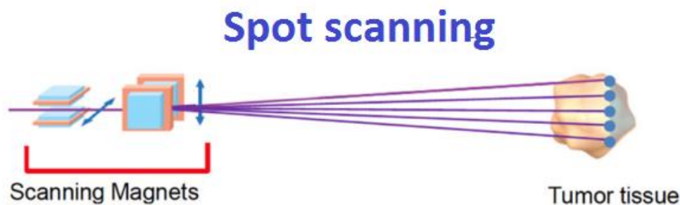
Figure 2.4: Active spot scanning proton therapy only uses magnets to guide the protons to the tumor. Modified from (Durante & Paganetti, 2016)
