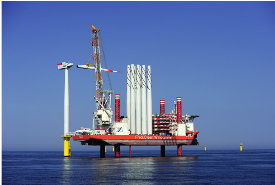
Figure 2.2.1.: Fred. Olsen's Bold Tern - a self-propelled jack-up vessel.
