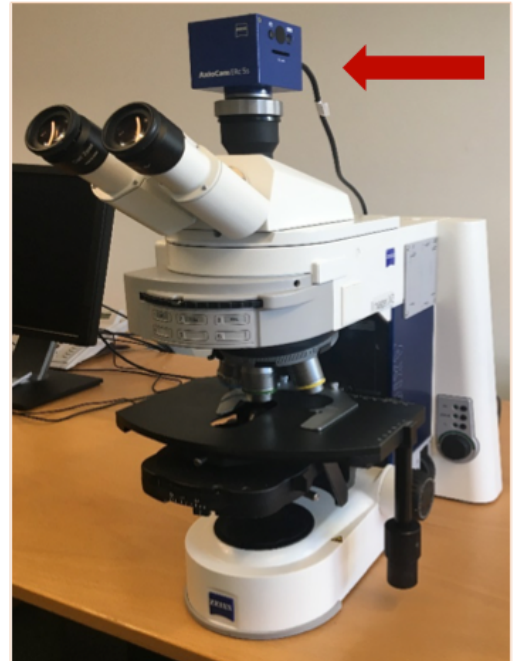
Figure 3. 4: The Zeiss Axioplan transmitted light microscope used to analyse the samples in this study. The AxioCam 5s camera used to capture all the images that were analysed is indicated with a red arrow.
