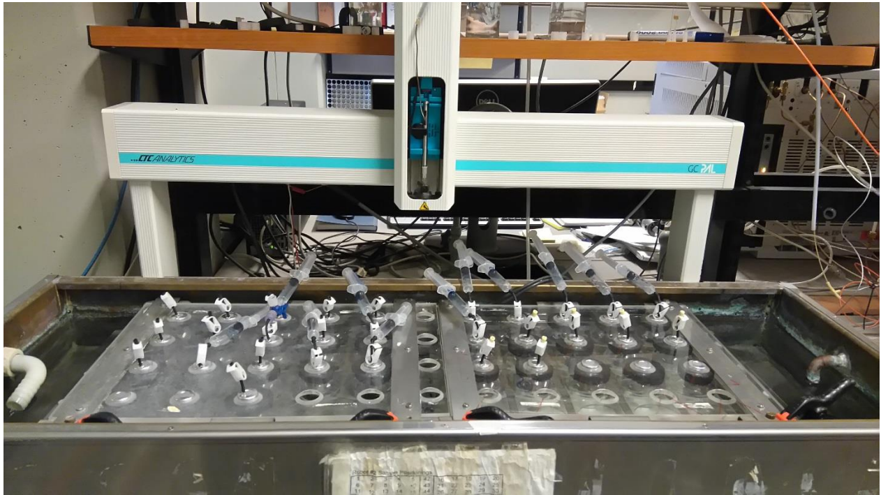
Figure 2.7: Placement of incubation bottles equipped with microrhizons in the incubator during the main experiment. Some of the bottles are being sampled for soil water through attached syringes.
