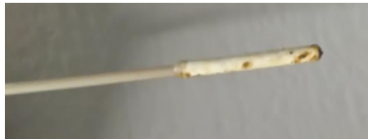
Figure 3.7: Microrhizon after second pilot experiment, with fine particles on the outside of the membrane.
