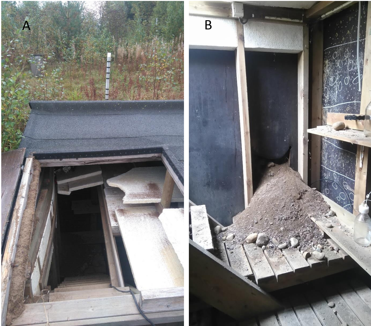
Figure 2.1: A: The prebuilt research trench at Moreppen research station, located at 60^{\circ}13'06.5208''\text{N} , 11^{\circ}05'15.2268''\text{E} , photo G. Flatabø September 14 th 2016. The door is normally closed to prevent precipitation and animals from entering the trench. B: A hole made in the east wall of the trench. The cover had fallen off, so some soil had collapsed into the trench. The exposed soil was removed prior to sampling. The drawings on the right hand side depicts the geology of the soil profile behind the wall.
