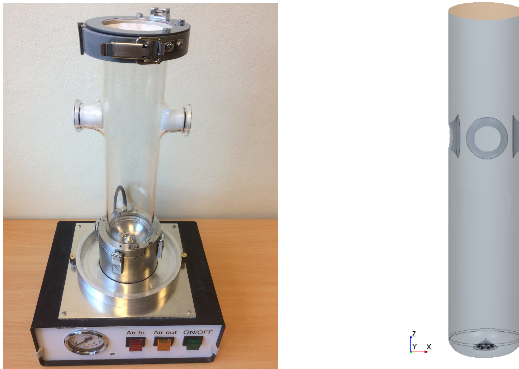
Figure 5: Left: Hartmann tube used in experiments. Right: CAD-model of the geometry used in the simulations.
