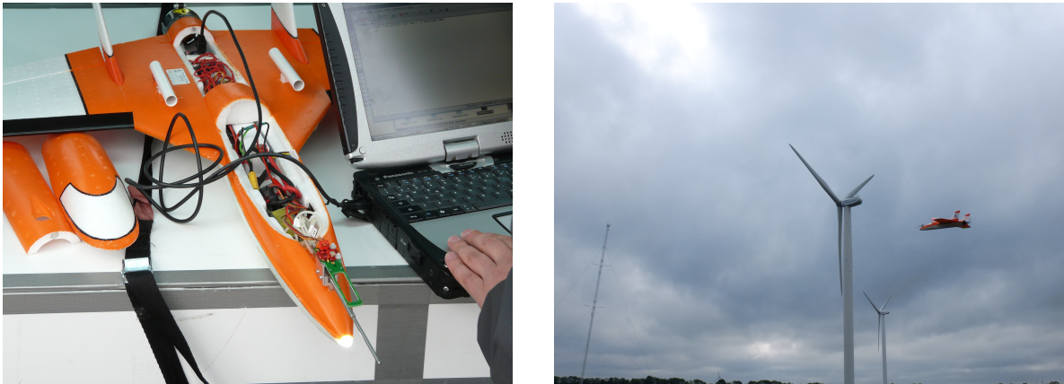
Fig. 1. The left picture shows the SUMO system during the initialization before start. The five-hole flow probe for turbulence measurements is the grey tube mounted on the nose of the airframe. The smaller green frame above is a fast-response fine-wire temperature sensor that has been flown for test purposes. The picture on the right shows SUMO in operation in front of two of the NORDEX N80 2.5 MW test turbines. The 108 m meteorological mast can be seen in the lower left corner of this picture.
