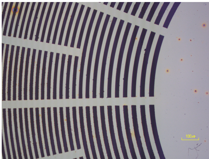
Figure 6.10: Optical reflective micrograph of the chromium zone plate. The dark is areas where the chrome layer has been removed.
