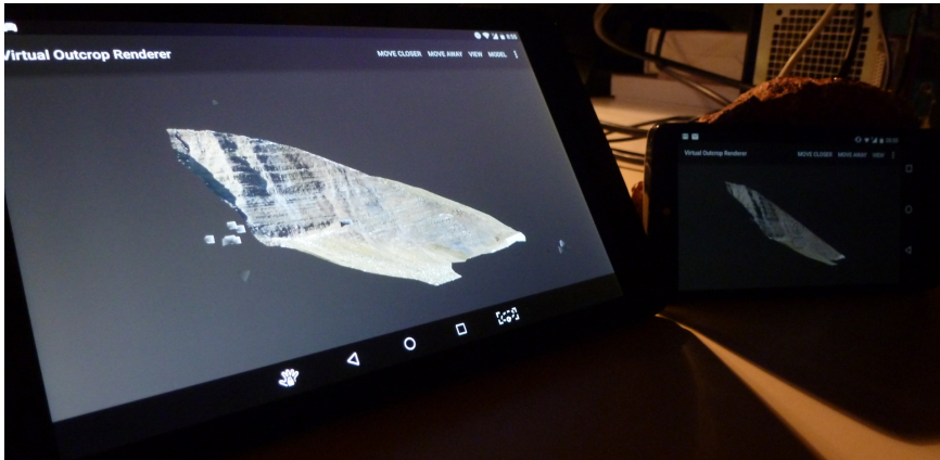
Figure 8.1: Proof of concept, showing the rendering of digital outcrops on tablets and smartphones directly on the device.
