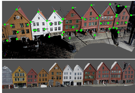
Figure 5: Rendering of the Bryggen dataset as coloured point set (top) and textured surface model (bottom), stretching along 40 m laterally. The green markers (top) highlight 3D control points for manual registration procedures.
