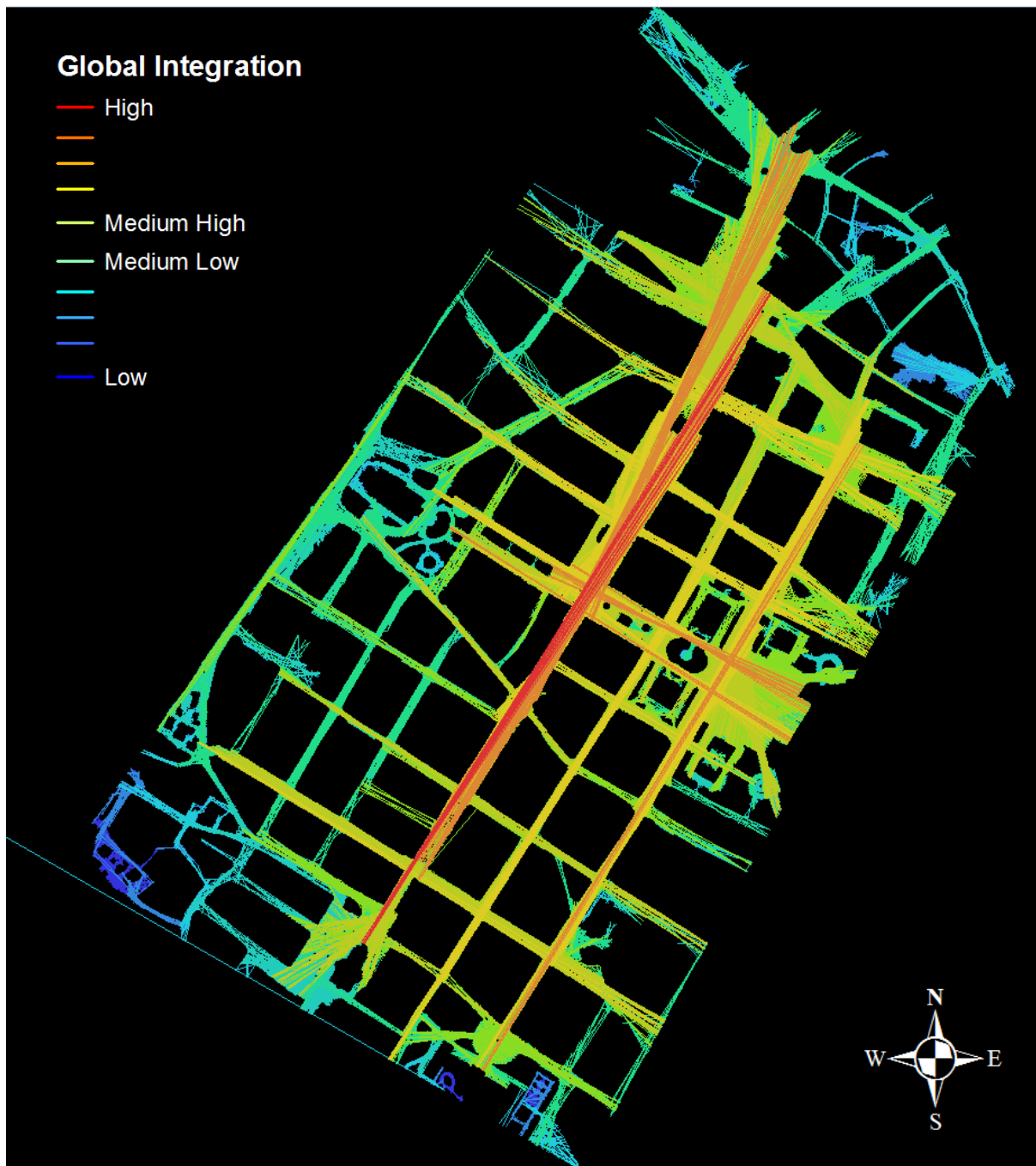
Figure 4-7: Global integration on all-line of Torgalmenningen axis. In convex spaces like Festplassen this analysis shows all possible walking paths and their potential attractivity..
