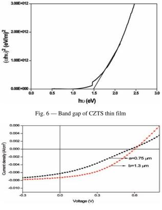
Fig. 7 — J - V characteristics of CZTS thin film solar cells
