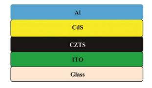
Fig. 1 — Schematic diagram of CZTS thin film based solar cell
