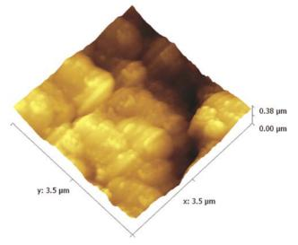
Fig. 3 — Atomic force micrograph of CZTS thin film
