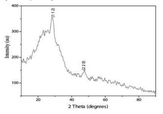
Fig. 2 — X-ray diffraction pattern of CZTS thin film
