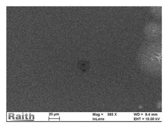
Fig. 4 — SEM image of CZTS thin film
