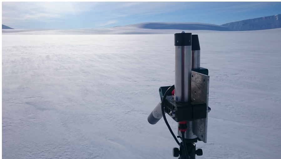
Figure 3.3: Photos from Kongsvegen, April 13th, 2016, showing an overview of the whole radiometer setup (top), and a close up (bottom). The two irradiance sensors are mounted to a metallic plate in equal height, while the radiance sensor is facing the ground in a 45^\circ angle, pointing towards the solar azimuth angle. We used this scheme for all samplings on Svalbard in April 2016.
