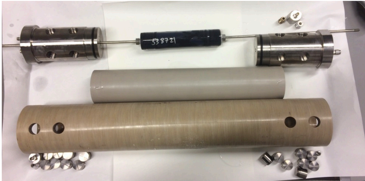
Figure 5-3: Picture of disassembled core holder. The core is mounted in the rubber sleeve and ready to use.
