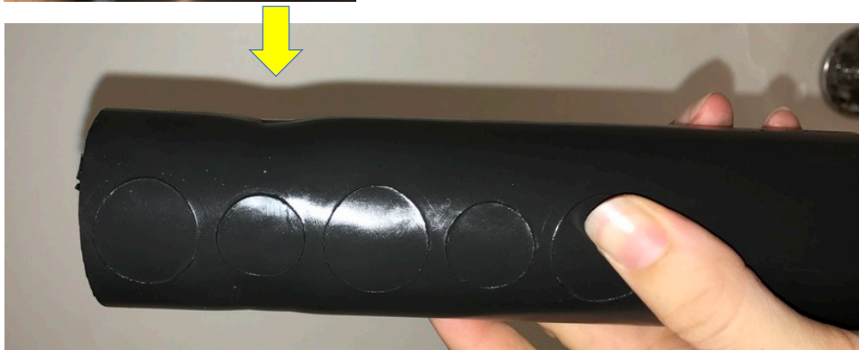
Figure C-1: Top: Illustration of the core holder, and the possible movement of the core in the sleeve mounted with the end-pieces. Below: images of the core in the sleeve. Left image show a fractured sleeve, and right a whole sleeve. Bottom image show where the end-piece had been moved out some, leading to the fracture in the sleeve.
