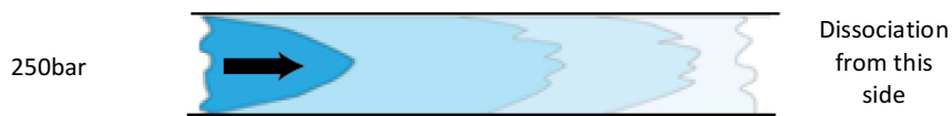
Figure 1: Illustration of a hydrate plug (blue) in a pipeline. In a scenario where the pressure is reduced in one end, the plug can melt and turn into a projectile (darker blue). This can cause damage on equipment, and in worst case scenarios result in fatal accidents.
