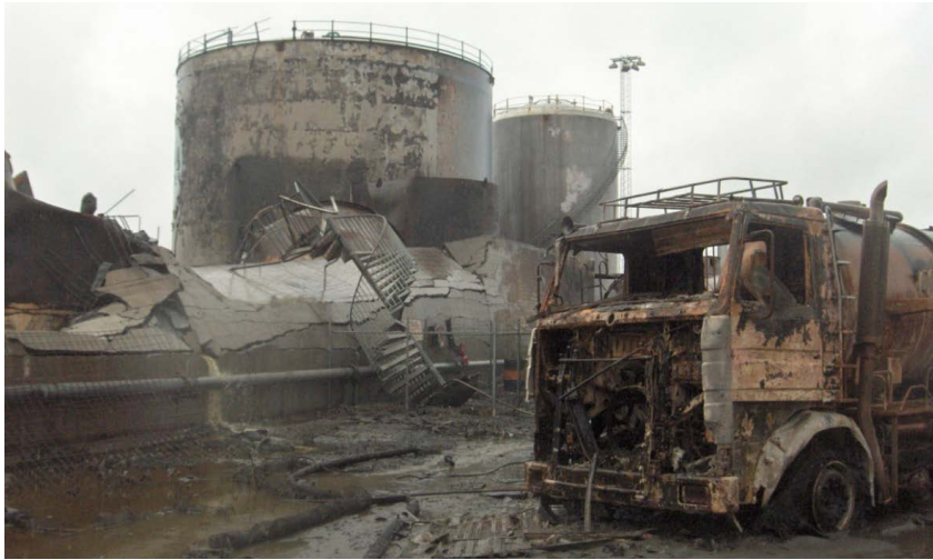
Figure 4: The accident caused severe damage in the industrial area, and the tank truck that delivered the hydrochloric acid was completely destroyed in the subsequent fire. Photo taken approximately six hours after the first explosion. Photo: Karl Otto Nesdal, Bergen brannvesen [Bergen Fire Department].
