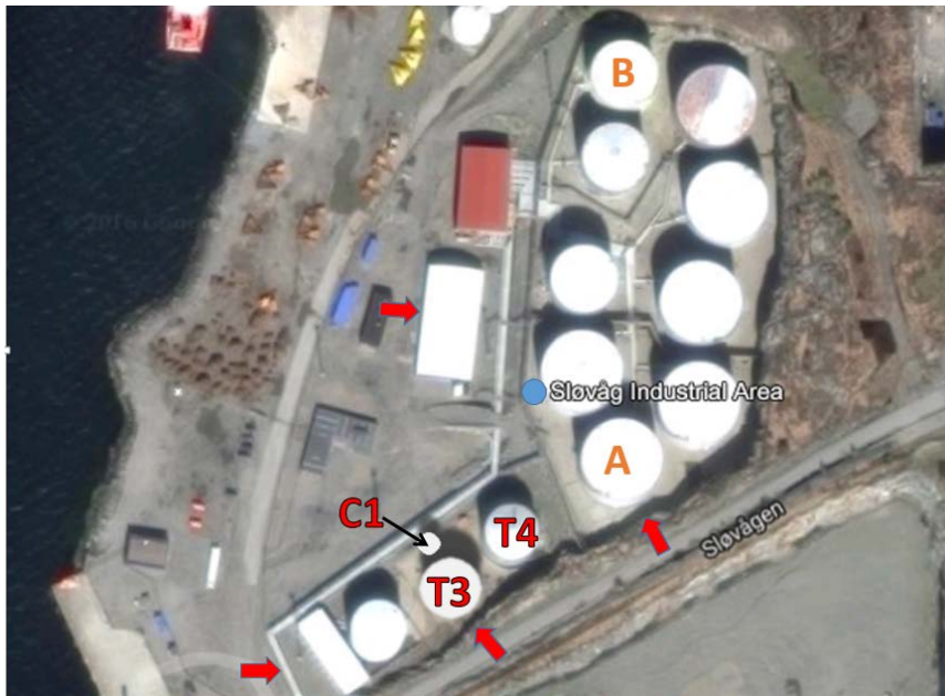
Figure 7: Manipulated satellite photo of the tank area. The three tanks that exploded in the accident, tanks T3, T4 and C1, are indicated. Sampling points for air measurements in 2007 (red arrows) and in 2008 (A and B) are also indicated. Satellite photo: Google Maps.
