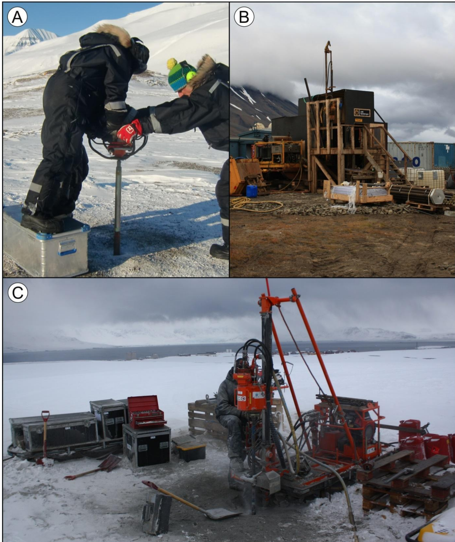
Figure 1. The different drilling infrastructure. A – Hand Drilling; B – Industrial Drill Rig; C – UNIS Permafrost Drill Rig.
