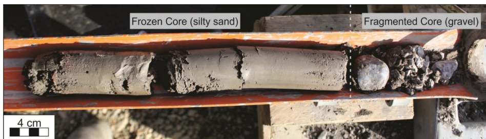
Figure 5. Differentiation between frozen and unfrozen, fragmented core retrieved using the UNIS Permafrost Drill Rig. Upwards direction is towards the left of the image.
