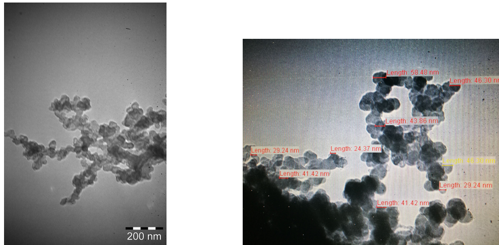
Figure 3.2: TEM pictures of CB NPs.
