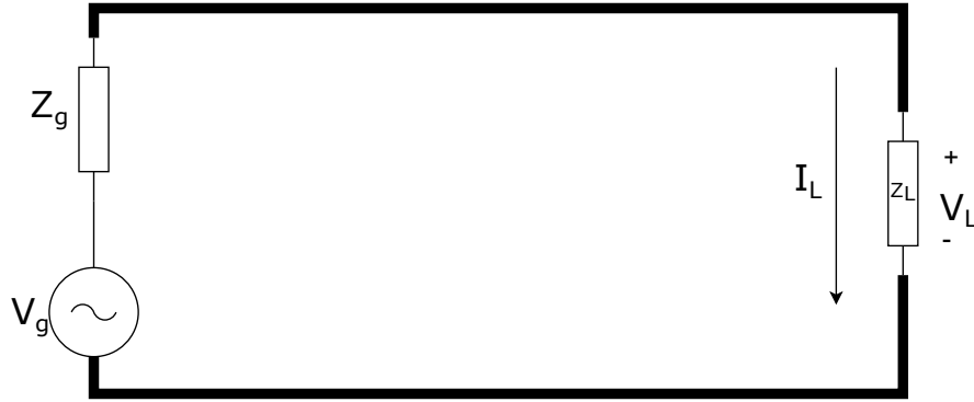
FIGURE 2.5: Transmission line with load.
