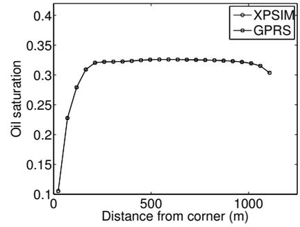
Figure 8: Oil saturation solution along diagonal from gridblock (1,1,1) to gridblock (24,24,1), Case 2a.
