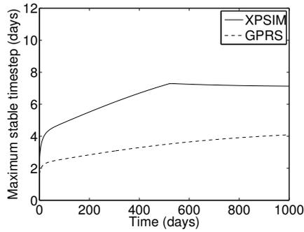
Figure 1: Predicted maximum stable timesteps during the simulation run of Case 1a, as calculated by (24) and (27).
