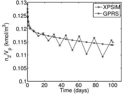
Figure 6: Detected instability, Case 2a, using a CFL factor of 2.0 in (26).
