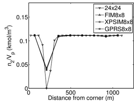
**Figure 14: Normalized component amount along grid diagonal, Case 2a: Reference solution from block (1,1,1) to block (24,24,1) on a  $24 \times 24 \times 1$  grid, fully implicit solution (FIM) and IMPSAT solutions with XPSIM and GPRS from block (1,1,1) to block (8,8,1) on a  $8 \times 8 \times 1$  grid.**
