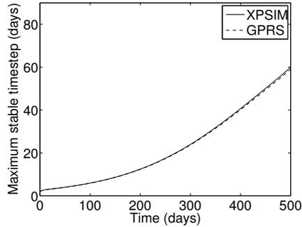
Figure 2: Predicted maximum stable timesteps during the simulation run of Case 2a, as calculated by (24) and (27).
