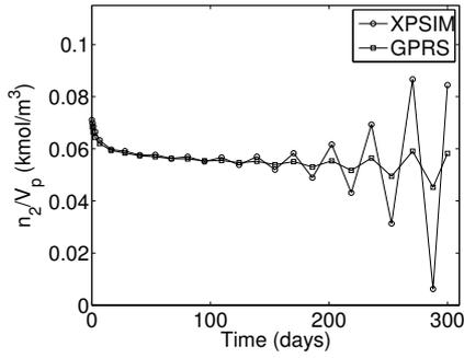
Figure 5: Detected instability, Case 1a, using a CFL factor of 3.0 in (26).
