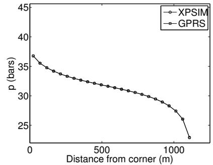
Figure 7: Pressure solution along diagonal from gridblock (1,1,1) to gridblock (24,24,1), Case 1a.
