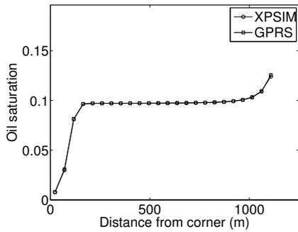
**Figure 11: Oil saturation solution along diagonal from gridblock (1,1,1) to gridblock (24,24,1), Case 2a.**
