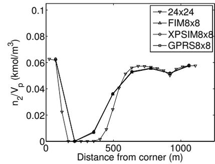
**Figure 13: Normalized component amount along grid diagonal, Case 1a: Reference solution from block (1,1,1) to block (24,24,1) on a  $24 \times 24 \times 1$  grid, fully implicit solution (FIM) and IMPSAT solutions with XPSIM and GPRS from block (1,1,1) to block (8,8,1) on a  $8 \times 8 \times 1$  grid.**
