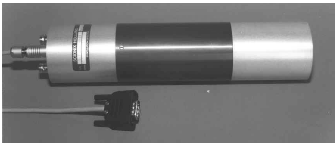
Figure B.1 Scionix 51B51/2-HV-EP scintillation detector with integrated high voltage power supply and charge sensitive preamplifier.
