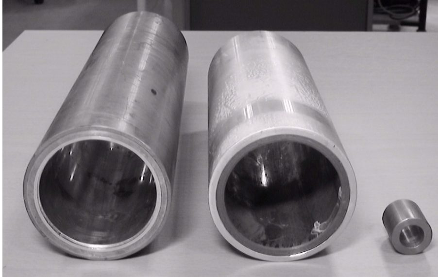
Figure A.5 Detector shields. Left: Three layer shield (Pb, Cu and Sn) for the scintillation detector. Middle: Two layer shield (Al and Pb) for the scintillation detector. Right: Lead shield for the semiconductor detector.
