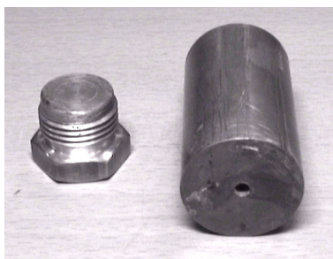
Figure A.1 Collimator for absolute fluorescence yield measurements.
