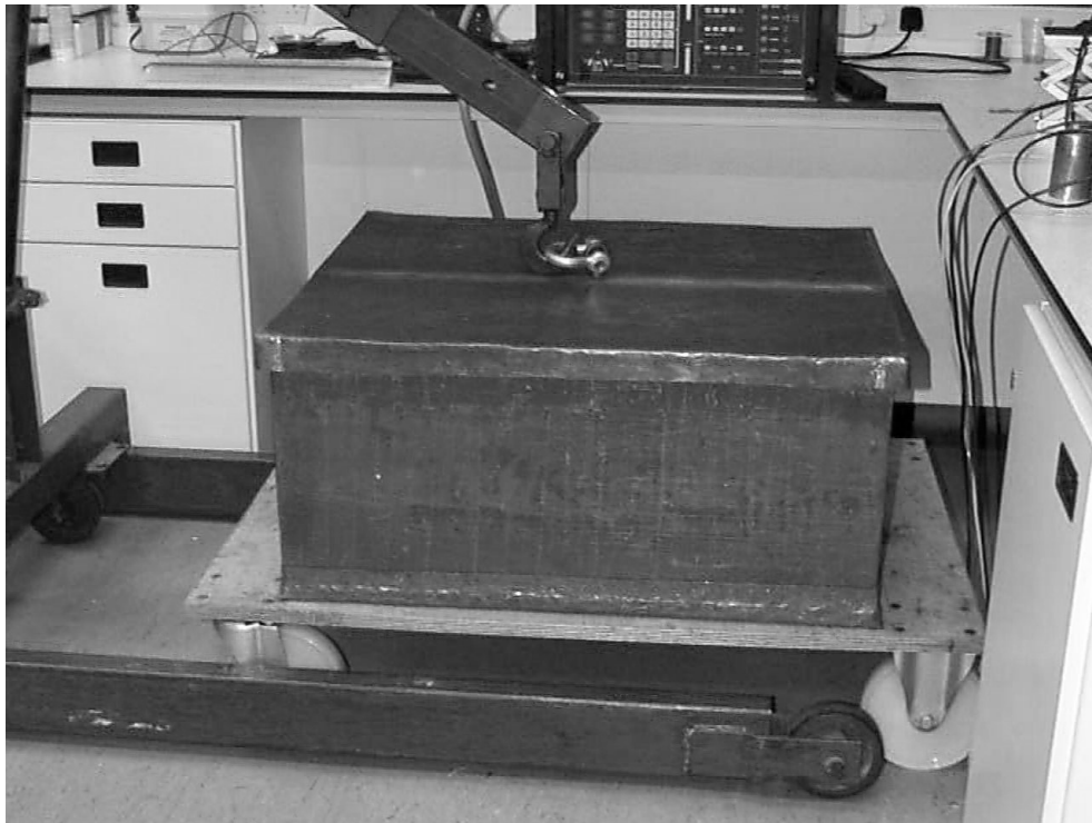
Figure A.6 Lead enclosure, exterior.
