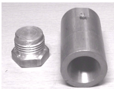
Figure A.2 Collimator for relative fluorescence yield measurements, with source above the sample surface.
