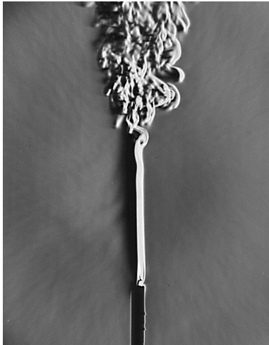
Figure 2.5: The plume from an ordinary candle transitions from laminar to turbulent flow, from Wikipedia [20].
