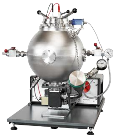
Figure 3.1: 20-liter explosion chamber, from Cesana-AG [37].
