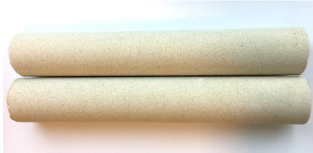
Figure 7.1 – 2" homogeneous Bentheimer sandstone core plugs
