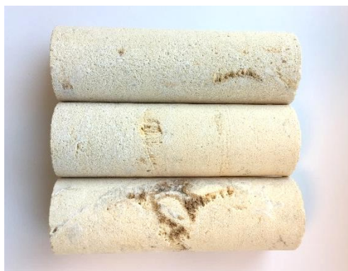
Figure 7.2 – 2" diameter Edwards limestone core plugs displaying heterogeneity
