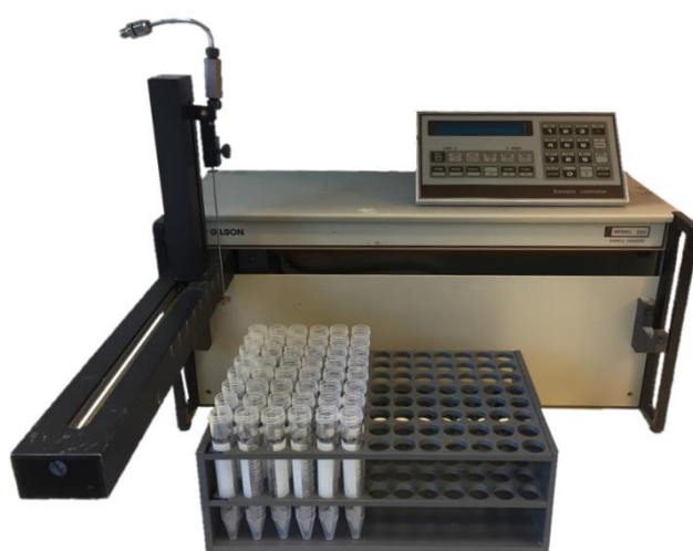
Figure 7.6 – Fractional collector controlling the production and tray with plastic vials to collect production.
