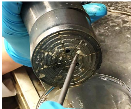
Figure 11.2 – NPA aggregates at inlet end-piece during adsorption test on EDW03. Aggregation generated a “gel” of nanoparticles at the inlet end-piece.
