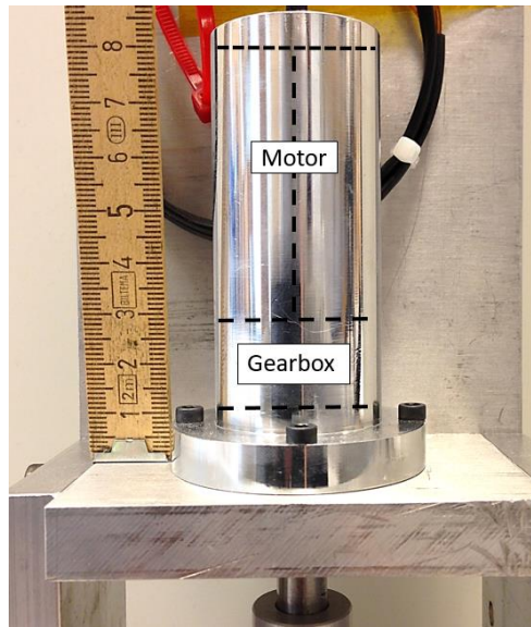
Figure 5. Phytron phySPACE stepper motor. Mounted on the frame used during development. Motor height, approximately 8 cm.
