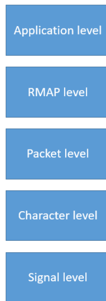
Figure 9. RoR protocol stack. The RoR communication protocol which the E-box modules must follow, including the RSE, contains five hierarchical levels.
