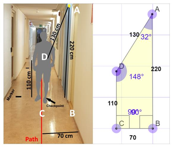
Figure 6.2: Illustration showing the measurements at the point closest to the beacon
