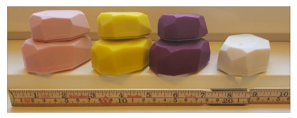
Figure 3.1: The location beacons from Estimote, the ones with UWB at the bottom
