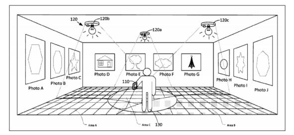
Figure 3.8: Image from Google's patent on an IPS using LiFi technology
