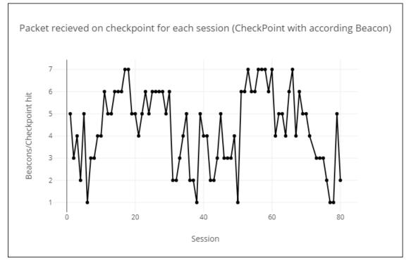
Graph 6.8: Graph that shows the hit rates for adjacent beacon's signal on the checkpoints
