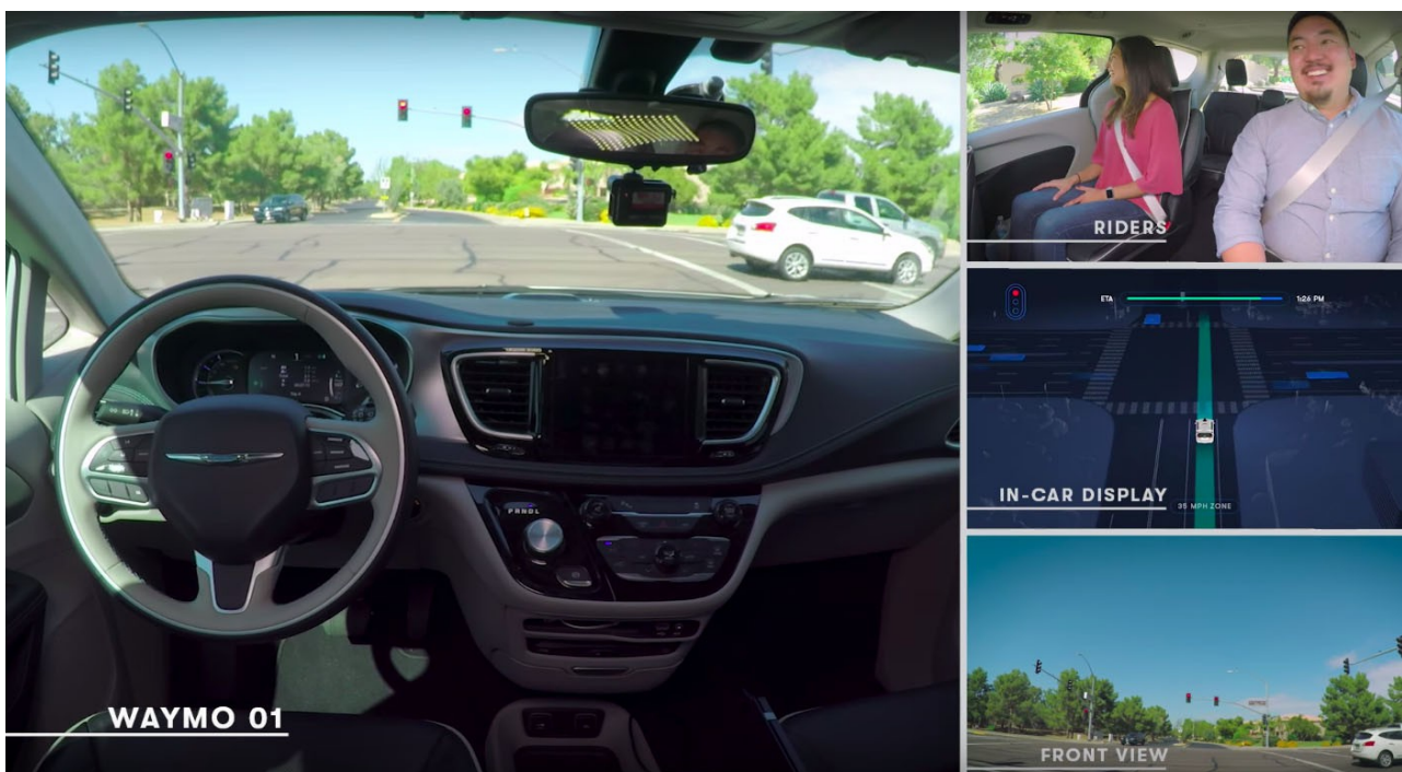
Illustration 5: Interior of Waymo's AV, showing empty driver's seat, riders in the backseat, and in-car display updating riders about vehicles intentions. (Copyright Waymo. 2018)
