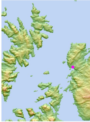
Figure 3: A 100 m model topography of the Melkøya area. The magenta dot indicates Hammerfest. Melkøya is the small island northwest of this town. The panel is useful in understanding how the topography influences the wind at Melkøya.
