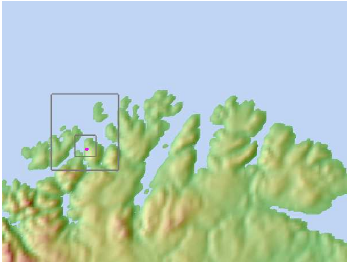
Figure 2: The MC2 3km 1km and 250m domains, respectively. The magenta dot indicates Hammerfest, the town southeast of Melkøya.
