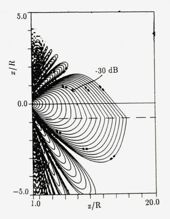
FIG. 4.12. Sound pressure amplitude, uniform source, ka = 10,  $\bar{\alpha}L_H = 0.1$ .  $c_0 =$  Profile 2,  $x_c = -4.0$ ,  $\theta = 75^{\circ}$ ,  $AL_H = 0.5$ .  $\Delta dB = 2$ .
