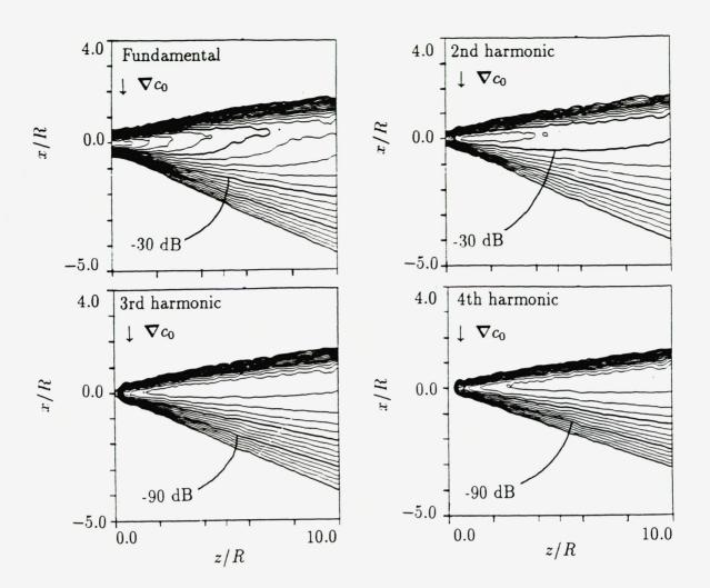
FIG. 5.8. Gaussian source, fully nonlinear case,  $R/l_d = 0.25$ ,  $R\bar{\alpha} = 0$ .  $c_0 =$  Profile 11,  $\theta = 90^{\circ}$ ,  $x_c = 0$ . Fundamental:  $\Delta dB = 3$ , higher harmonics:  $\Delta dB = 6$ .
