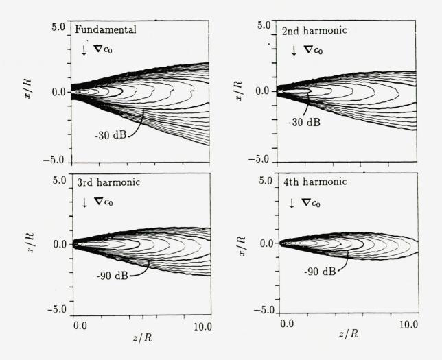
FIG. 5.12. Gaussian source, fully nonlinear case,  $R/l_d = 0.25$ ,  $R\bar{\alpha} = 0.1$ .  $c_0 =$  Profile 2,  $\theta = 90^{\circ}$ ,  $x_c = 0$ . Fundamental:  $\Delta dB = 3$ , higher harmonics:  $\Delta dB = 6$ .
