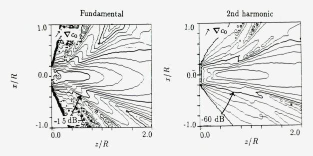
FIG. 5.10. Uniform source, quasilinear case,  $R/l_d = 0.05$ ,  $R\bar{\alpha} = 0$ .  $c_0 = \text{Profile 1}$ ,  $\theta = 75^\circ$ ,  $x_c = 0$ . Fundamental:  $\Delta dB = 3$ , second harmonic:  $\Delta dB = 6$ .
