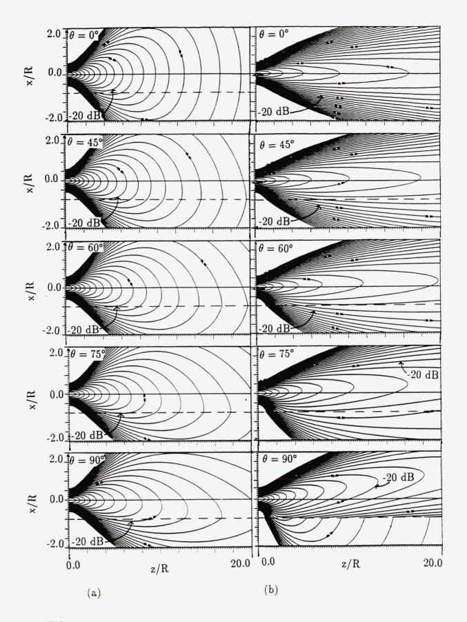
FIG. 4.5. Sound pressure amplitudes for various  $\theta$  and sound speed profiles. Gaussian source,  $x_c = -4.0$ , ka = 10, no absorption.  $\theta = 0^{\circ}$ , 45°, 60°, 75°, 90°,  $AL_H = 0.1$ . (a)  $c_0 =$  Profile 1. (b)  $c_0 =$  Profile 2.  $\Delta dB = 2$ .
