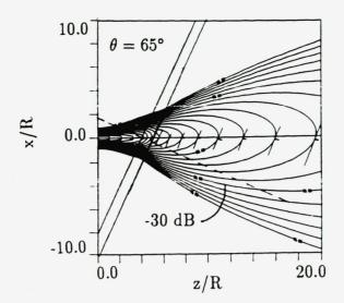
FIG. 4.19. Continuous interface simulation, amplitude: ka = 10,  $a = 2\bar{a}$ ,  $\theta = 65^{\circ}$ .  $c_2/c_1 = 2.0$ .  $\Delta dB = 2$ .
