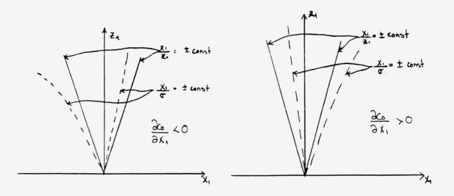
FIG. 4.2. Bending of the lines x/z = constant due to inhomogeneity.
