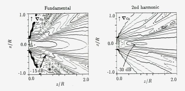
FIG. 5.4. Uniform source, quasilinear case,  $R/l_d = 0.05$ ,  $R\bar{\alpha} = 0$ .  $c_0 =$  Profile 22,  $\theta = 90^{\circ}$ ,  $x_c = 0$ . Fundamental:  $\Delta dB = 3$ , second harmonic:  $\Delta dB = 6$ .
