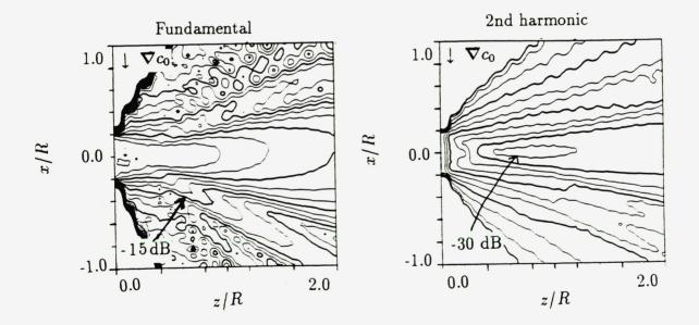
FIG. 5.3. Uniform source, quasilinear case,  $R/l_d = 0.05$ ,  $R\bar{\alpha} = 0$ .  $c_0 =$  Profile 2,  $\theta = 90^{\circ}$ ,  $x_c = 0$ . Fundamental:  $\Delta dB = 3$ , second harmonic:  $\Delta dB = 6$ .
