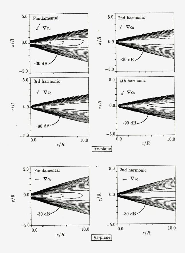
FIG. 5.9. Gaussian source, fully nonlinear case,  $R/l_d = 0.25$ ,  $R\bar{\alpha} = 0$ .  $c_0 =$  Profile 2.  $\theta = 75^{\circ}$ ,  $x_c = 0$ . Fundamental:  $\Delta dB = 3$ , higher harmonics:  $\Delta dB = 6$ .
