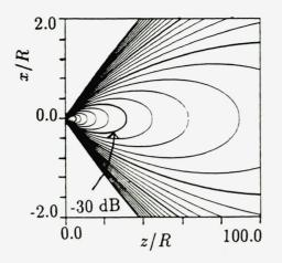
FIG. 4.9. Sound pressure amplitude radiated from Gaussian source, homogeneous, nondissipative case, ka = 100.
