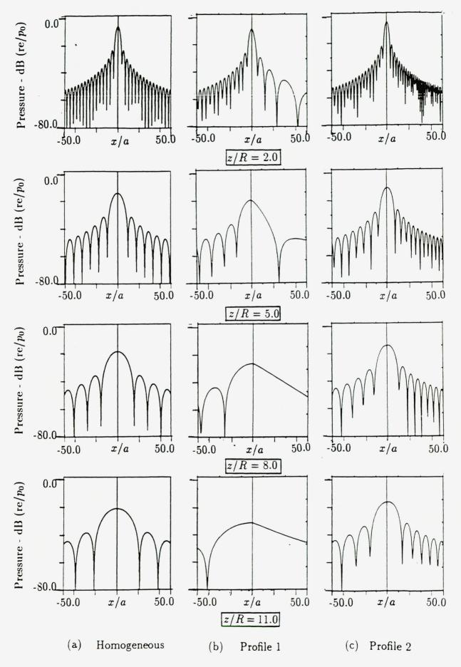
FIG. 4.3. Beampatterns. Uniform piston source, ka = 20. (a) Homogeneous medium. (b)  $c_0$  = Profile 1. (c)  $c_0$  = Profile 2.  $AL_H = 0.5$ ,  $\theta = 70^\circ$ ,  $x_c = 0.0$ , no absorption in all cases. z/R = 2.0, 5.0, 8.0, 11.0.
