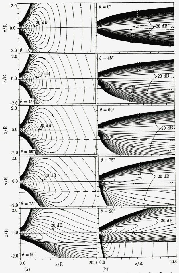
FIG. 4.6. Sound pressure amplitudes for various  $\theta$  and sound speed profiles. Gaussian source,  $x_c = -4.0$ , ka = 10, no absorption.  $\theta = 0^{\circ}$ , 45°, 60°, 75°, 90°,  $AL_H = 1.0$ . (a)  $c_0 = \text{Profile 22.}$  (b)  $c_0 = \text{Profile 11.} \Delta dB = 2$ .
