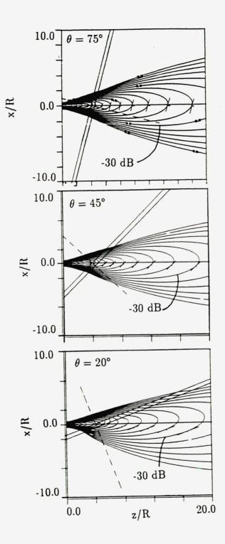
FIG. 4.17. Continuous interface simulation, amplitude: varying  $\theta$ , fixed ka.  $c_2/c_1 = 1.5$ .  $\theta = 75^{\circ}$ , 45°, 20°.  $\Delta dB = 2$ .
