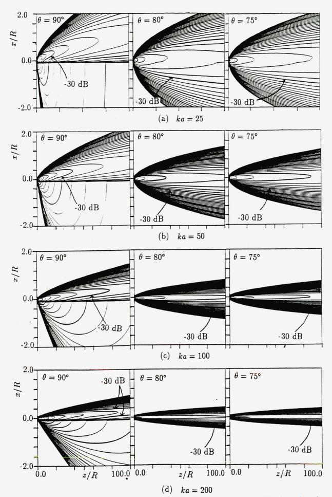
FIG. 4.10. Various ka: fixed a and various k. Sound pressure amplitude radiated from Gaussian source.  $c_0$  = Profile 2,  $\theta$  = 90°, 80°, 75°. (a) ka = 25. (b) ka = 50. (c) ka = 100. (d) ka = 200.
