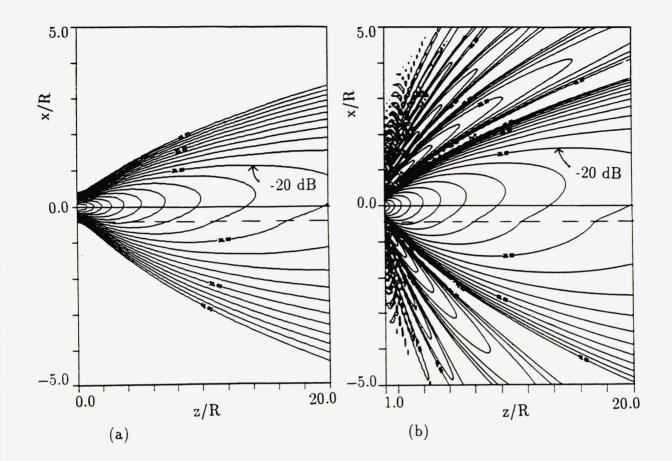
FIG. 4.4. Sound pressure amplitude.  $c_0$  = Profile 2,  $\theta = 75^{\circ}$ ,  $AL_H = 0.5$ ,  $x_c = -2.0$ , ka = 10, no absorption. (a) Gaussian source. (b) Uniform source.  $\Delta dB = 2$ .
