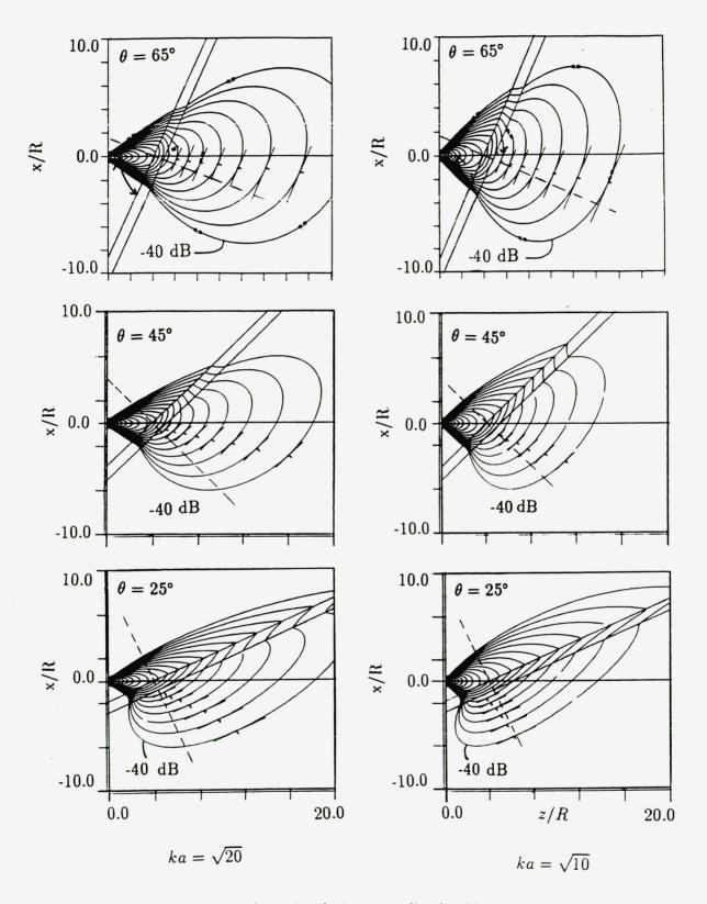
FIG. 4.18. Continuous interface simulation, amplitude: Varying k and fixed source radius.  $ka = 20^{1/2}$ ,  $ka = 10^{1/2}$ , for  $\theta = \theta = 65^{\circ}$ ,  $45^{\circ}$ ,  $20^{\circ}$ .  $c_2/c_1 = 2.0$ .  $\Delta dB = 2$ .
