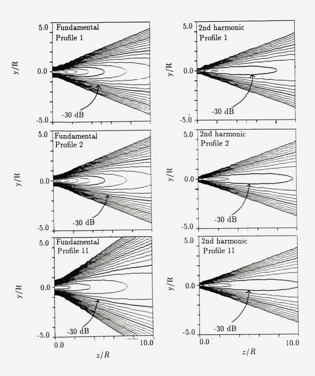
FIG. 5.11. Gaussian source, fully nonlinear case,  $R/l_d = 0.25$ ,  $R\bar{\alpha} = 0$ . Amplitude in the yz-plane, where there is no transverse component of  $\nabla c_0$ .  $\theta = 90^\circ$ ,  $x_c = 0$ . Fundamental:  $\Delta dB = 3$ , higher harmonics:  $\Delta dB = 6$ .
