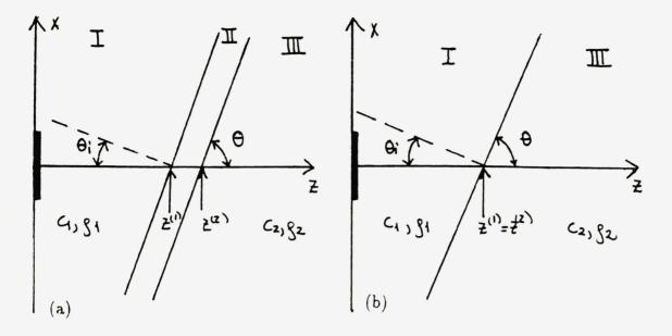
FIG. 4.14. Geometry of a fluid-fluid interface. (a) Case 1. (b) Case 2.
