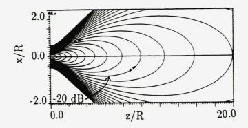
FIG. 4.7. Sound pressure amplitude,  $\nabla c_0 = 0$ , ka = 10. Gaussian source, no absorption.  $\Delta dB = 2$ .
