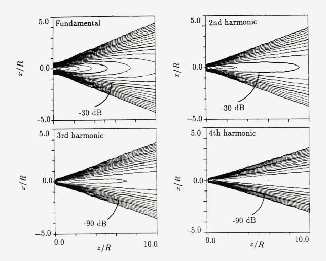
FIG. 5.5. Gaussian source, fully nonlinear case,  $R/l_d = 0.25$ ,  $R\bar{\alpha} = 0$ . Homogeneous, nondissipative medium. Fundamental:  $\Delta dB = 3$ , higher harmonics:  $\Delta dB = 6$ .
