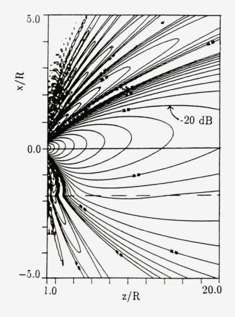
FIG. 4.8. Sound pressure amplitude, uniform source, ka = 10, no absorption.  $c_0 =$  Profile 2,  $\theta = 75^{\circ}$ ,  $AL_H = 0.5$ ,  $x_c = -9.0$ .  $\Delta dB = 2$ .
