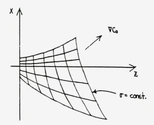
FIG. 3.1. Curved coordinate mesh used in the numerical calculations.
