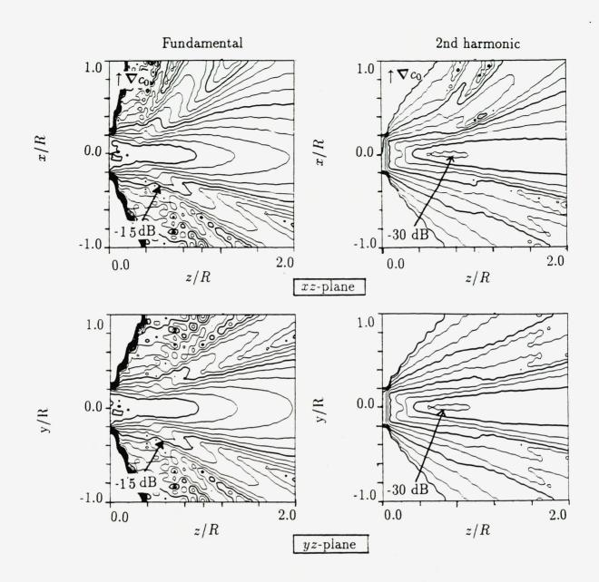
FIG. 5.1. Uniform source, quasilinear case,  $R/l_d = 0.05$ ,  $R\bar{\alpha} = 0$ .  $c_0 =$  Profile 1,  $\theta = 90^{\circ}$ ,  $x_c = 0$ . Fundamental:  $\Delta dB = 3$ , second harmonic:  $\Delta dB = 6$ .
