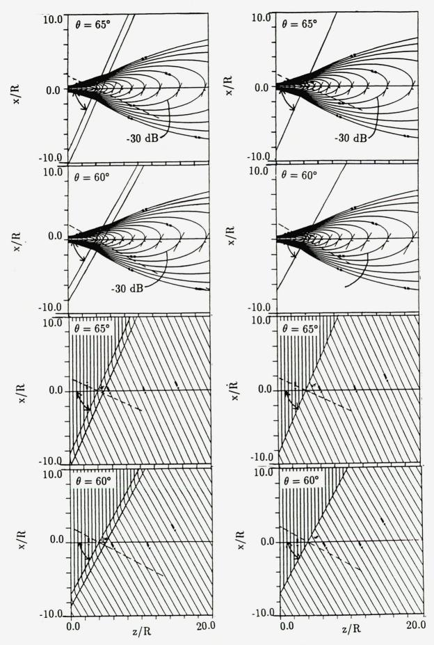
FIG. 4.16. Continuous vs. discontinuous simulation of interface. Amplitude and phase ( $\phi$ ).  $c_2/c_1 = 2.0$ .  $\theta = 60^{\circ}$ , 65°.  $\Delta dB = 2$ ,  $\Delta \phi = 50$ .
