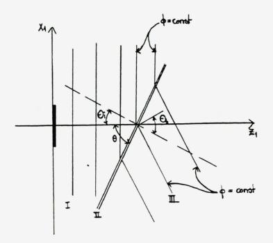
FIG. 4.15. The surfaces  $\phi = \text{constant}$  in fluid-fluid interface simulation.
