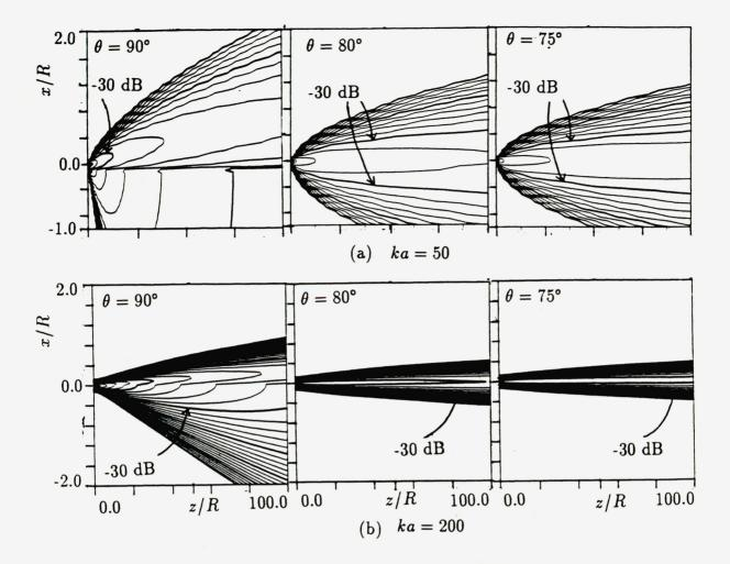
FIG. 4.11. Various ka: fixed k and various a. Sound pressure amplitude radiated from Gaussian source.  $c_0 = \text{Profile } 2, \theta = 90^{\circ}, 80^{\circ}, 75^{\circ}$ . (a) ka = 50. (b) ka = 200.
