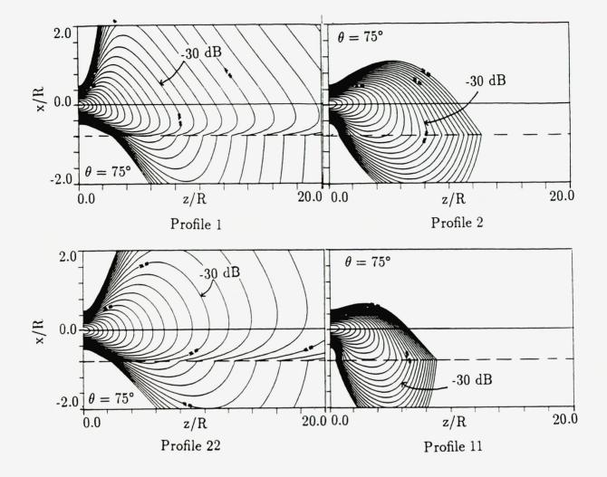
FIG. 4.13. Sound pressure amplitude, Gaussian source, ka = 10,  $\bar{\alpha}L_H = 0.1$ , for various soundspeed profiles.  $x_c = -4.0$ ,  $\theta = 75^\circ$ ,  $AL_H = 1.0$ .  $\Delta dB = 2$ .
