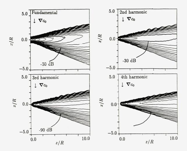
FIG. 5.7. Gaussian source, fully nonlinear case,  $R/l_d = 0.25$ ,  $R\bar{\alpha} = 0$ .  $c_0 =$  Profile 2,  $\theta = 90^{\circ}$ ,  $x_c = 0$ . Fundamental:  $\Delta dB = 3$ , higher harmonics:  $\Delta dB = 6$ .
