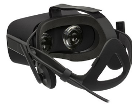
Figure 2.7: Oculus Rift CV1 HMD (Wikimedia Commons).[7]
