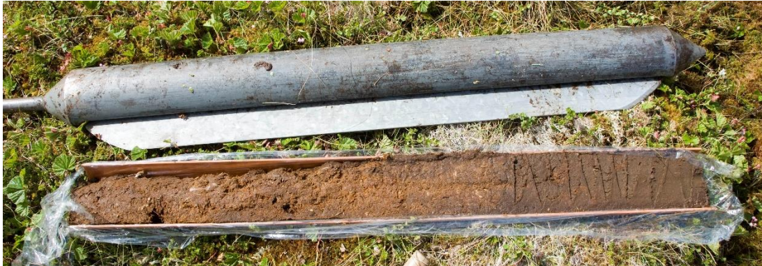
Figure 8: Peat sequences extracted from Stripåtmyrin using a 110 mm diameter Russian corer. Samples were sealed using plastic wrapping and duct tape.
