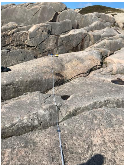
Figure 4.1-2 Linear scanline from the field locality Nesvika. The scanline is oriented approximately perpendicular to the dominating fracture set. Photo: Eirin Hermansen
