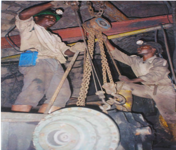
Fig. 5. A worker in underground maintenance repairing a winch (photograph by Simon H.D. Mamuya)
