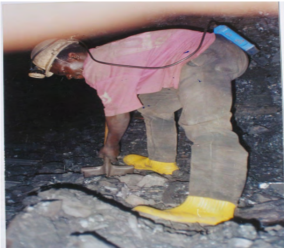
Fig. 4. Lashing coal in the mine team (photograph by Simon H.D. Mamuya)
