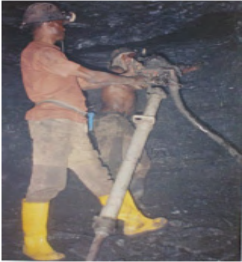
Fig. 3. Pneumatic drilling in development (photograph by Simon H.D. Mamuya)
