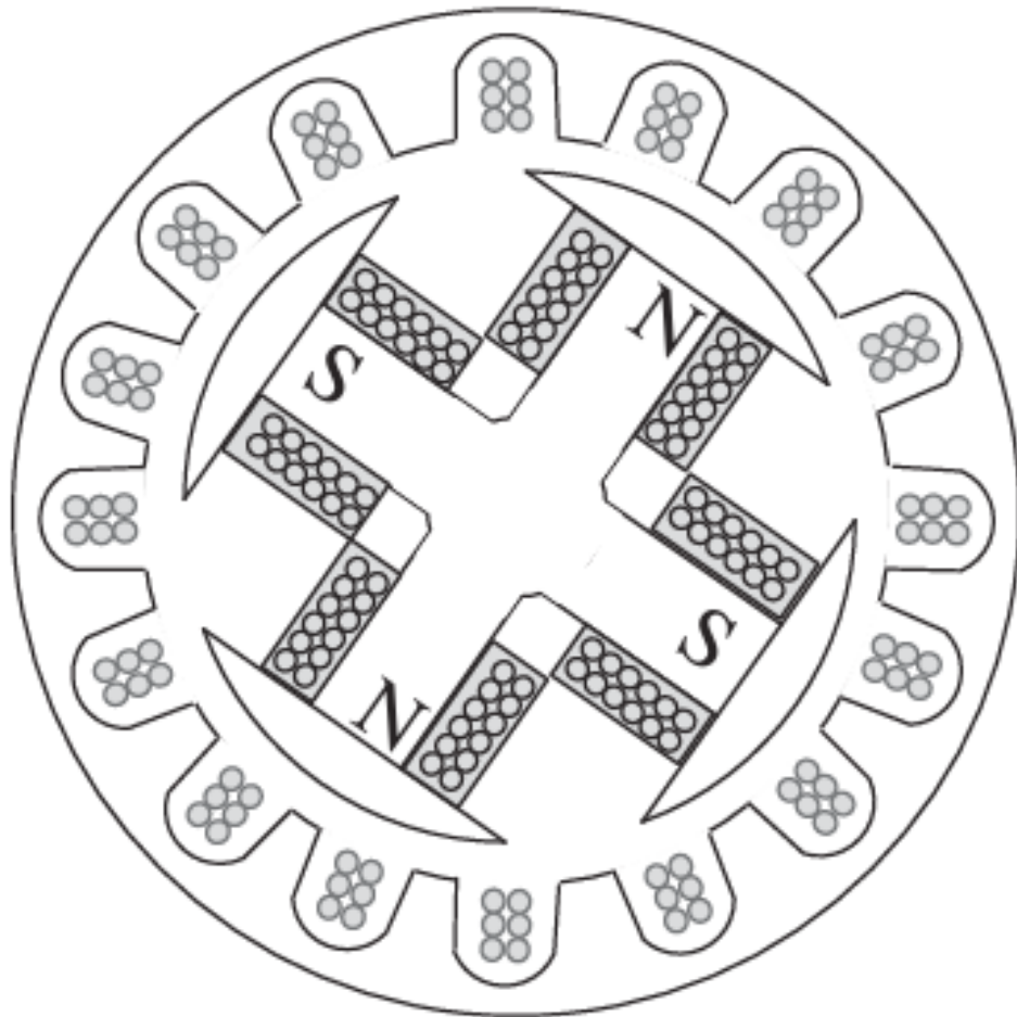
Figure 8: Cross-section of salient four-pole synchronous generator[17, p.74]
