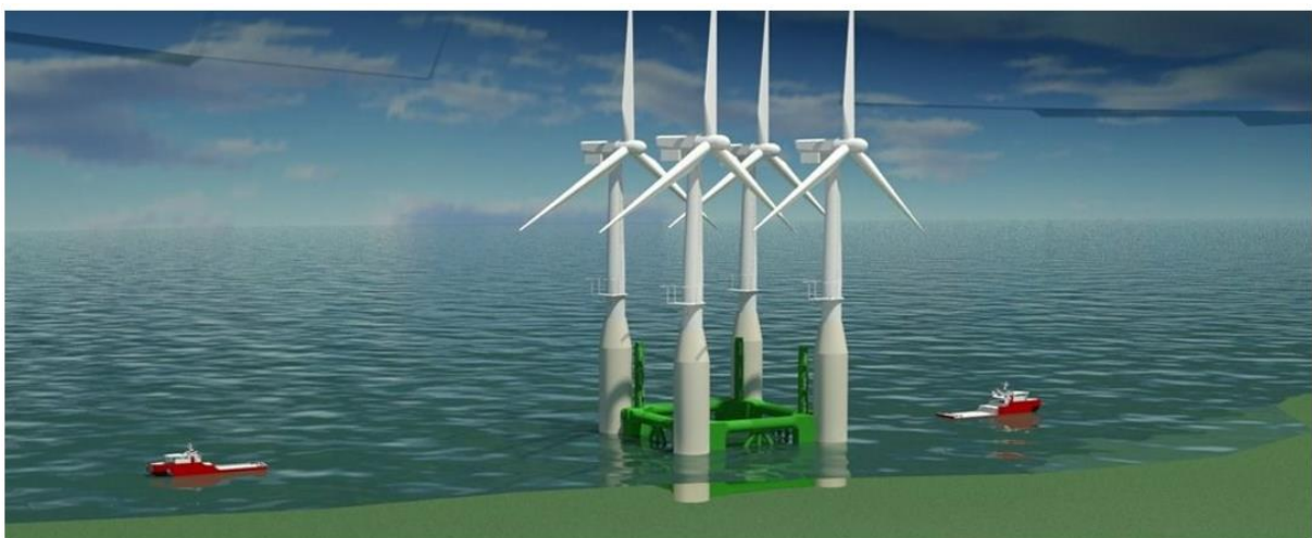
Figure 2 - The Atkins reusable transportation frame, allowing for multiple turbine transportation at reduced draft [5].
