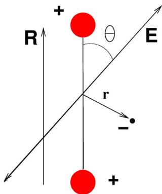
FIG. 1. (Color online) Coordinates (molecular frame); The protons are at a fixed distance  $R$  with the molecular axis defining the polar axis ( $z$  direction). The  $xz$ -plane is chosen so that it contains the polarization vector which defines an angle  $\theta$  with respect to the  $z$  axis. The electron coordinate, with its origin at the midpoint between the nuclei, is denoted by  $\mathbf{r}$ .
